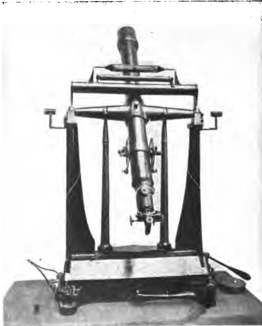
FIG. 86.—Large Portable Transit (Equipped with Transit Micrometer).
